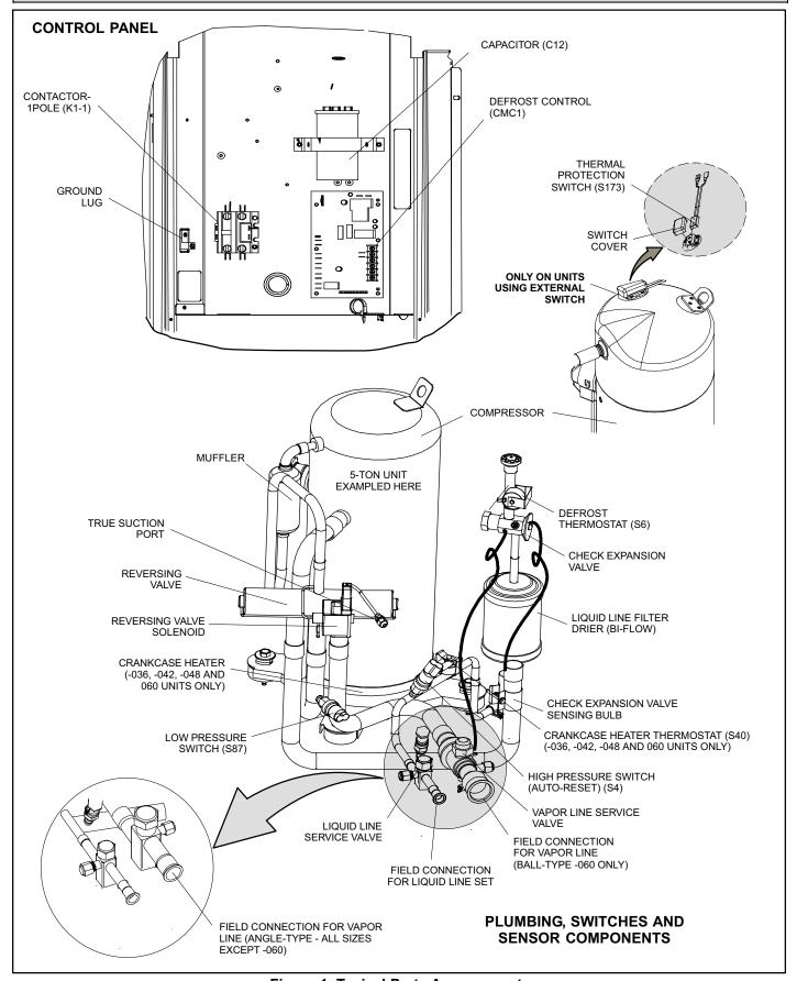
Figure 1. Typical Parts Arrangements
